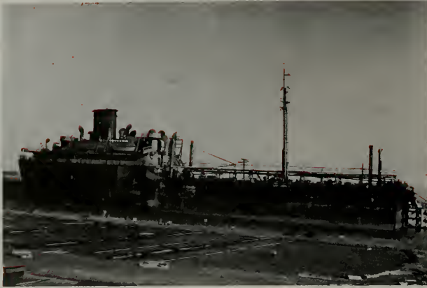
The SS Donbass, III, former Russian tanker which broke in two last February in the North Pacific, being operated by the Pacific Gas & Electric Company to augment the power supply of the fast-growing Humboldt area, by using the ship's main propulsion equipment.
